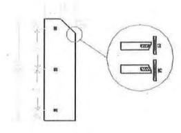
NOTE: Orders will be right-hand (R) or left-hand (L) to designate the direction of the taper on the leading edge.
