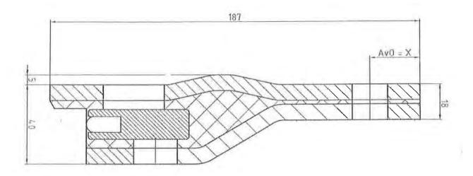
Figure 2: AASHTO Hole Positioning (4')
