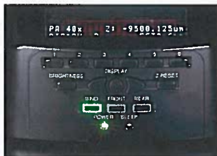
Figure 3. Controls are conveniently located on the front of the microscope base. Selected observation conditions can be designated to individual buttons, enabling changes to be made at the push of a button. This is particularly convenient when reproducing specific observation conditions.
